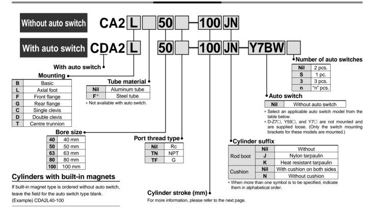
Applicable Auto Switch: Refer to Best Pneumatics ② for detailed auto switch specifications
