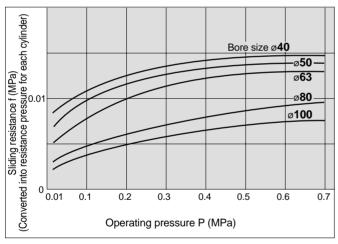
The actual sliding resistance F (N) can be found by the following equation from the sliding resistance f (MPa) (converted into resistance pressure of each cylinder) indicated by the ordinate of the graph.
