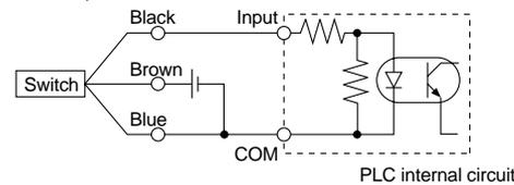
Connect according to the applicable PLC input specifications, as the connection method will vary depending on the PLC input specifications.
