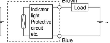
(Power supplies for switch and load are separate.)
