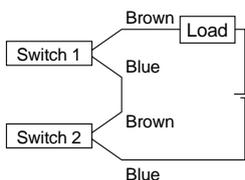
When two switches are connected in series, a load may malfunction because the load voltage will decline when in the ON state. The indicator lights will light when both switches are in the ON state.
