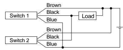
The indicator lights will light up when both switches are in the ON state.
