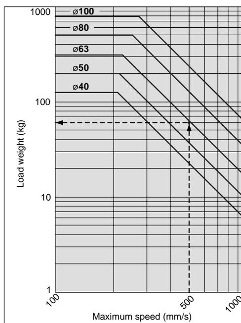
(Example) Find the upper limit of rod end load when an air cylinder of ø63 is operated at 500 mm/s.
