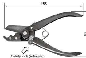
**TK-2** Applicable tubing O.D.: 18 mm or less
