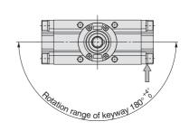
Note) If it is pressurised from the port indicated with the arrow, the shaft rotates in the clockwise direction.
