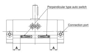
For size 30, only the perpendicular type auto switch can be mounted since two auto switches are mounted in the same switch groove when mounting the switch on the connection port side.
