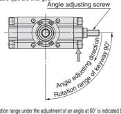
The rotation range under the adjustment of an angle at  $60^{\circ}$  is indicated below
