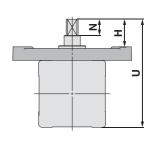
Single shaft with four chamfers: C□RA1FX
