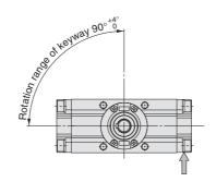
Note) If it is pressurised from the port indicated with the arrow, the shaft rotates in the clockwise direction.
