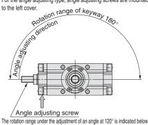
Rotation Pane Note) If it is pressurised from the port indicated with the arrow, the shaft rotates in the clockwise direc-
