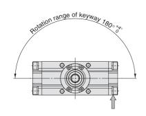
Note) If it is pressurised from the port indicated with the arrow, the shaft rotates in the clockwise direction.
