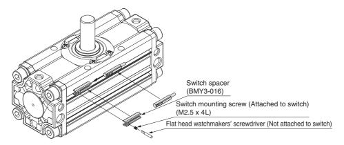
Note) When tightening an auto switch mounting screw, use a watchmakers' screwdriver with a handle of approximately 5 to 6 mm in diameter.
