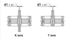
Shaft through-hole Note) Except flange type
