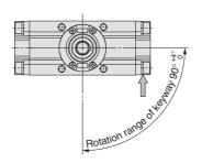
Note) If it is pressurised from the port indicated with the arrow, the shaft rotates in the clockwise direction.
