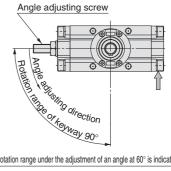
The rotation range under the adjustment of an angle at 60° is indicated below.
