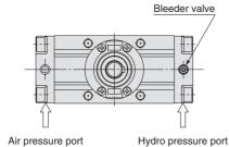
The figure shows the pressurised situation to the hydro pressure port.
