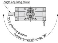
The rotation range under the adjustment of an angle at  $120^{\circ}$  is indicated below
