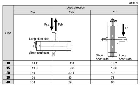
A load up to the allowable radial/thrust load can be applied provided that a dynamic load is not generated. However, applications which apply a load directly to the shaft should be avoided whenever possible. In order to further improve the operating conditions, a method such as that shown in the drawing below is recommended so that a direct load is not applied to the shaft.
