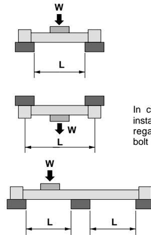
In case the product is installed on the ceiling, regard the mounting bolt pitch as L.
