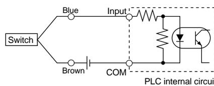
Connect according to the applicable PLC input specifications, as the connection method will vary depending on the PLC input specifications.
