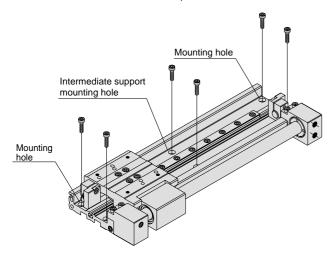
When a 25 mm adjustment bolt is selected, the mounting holes will be hidden behind it. Adjust the adjustment bolt after the cylinder is installed.
