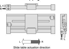
2. The plug position of the piping port can be changed to suit the operating conditions.
