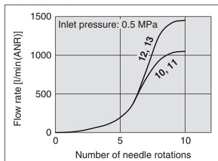
\* The numbers above the flow rate characteristic curves in the charts show the applicable tubing outside diameter as defined by the product number.
