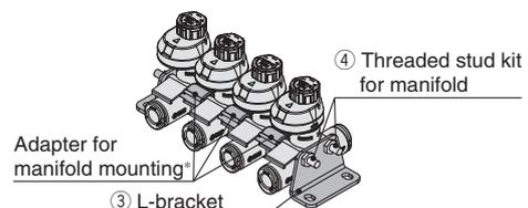
\* It is included in the threaded stud kit for manifold (excluding the AS4002FS□). Refer to the details of the kit shown on the left.
