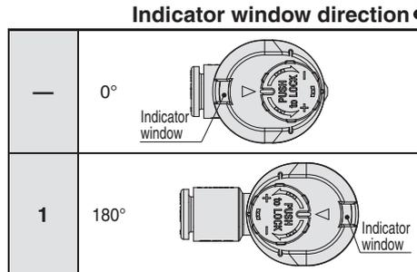
Note) Orientation of indicator direction is fixed when manufacturing, and cannot be changed by the user.
