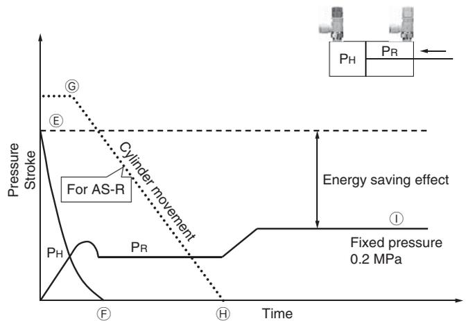
○ **Working stroke pressure/Stroke change**
