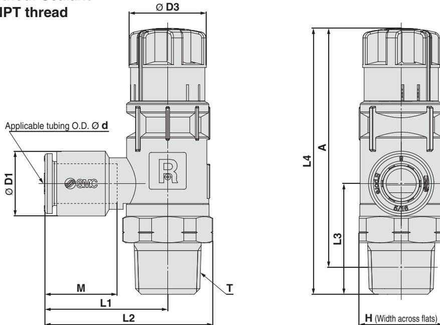
\* The release button of Ø 6 One-touch fitting is oval as shown above. The button can be rotated freely.
