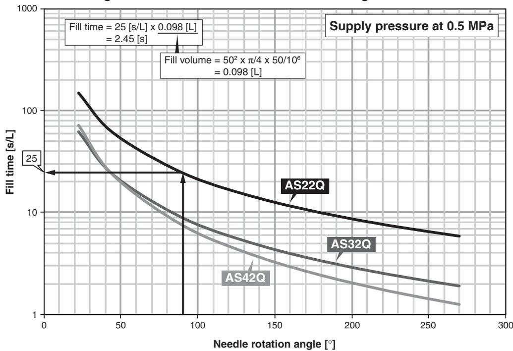
**Figure 2. Fill Time Diagram**
