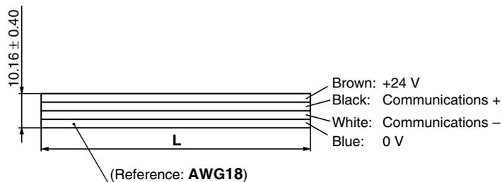
\* The maximum length of a branch cable for the EX510 series should be 20 metres or less.
