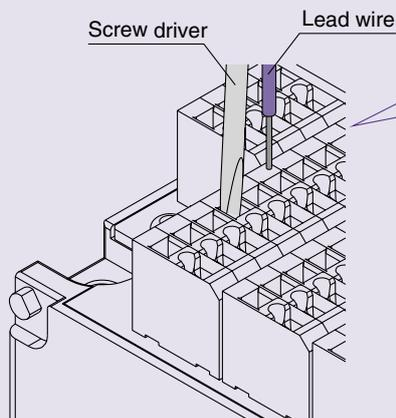
Torque control and crimping work is unnecessary.
