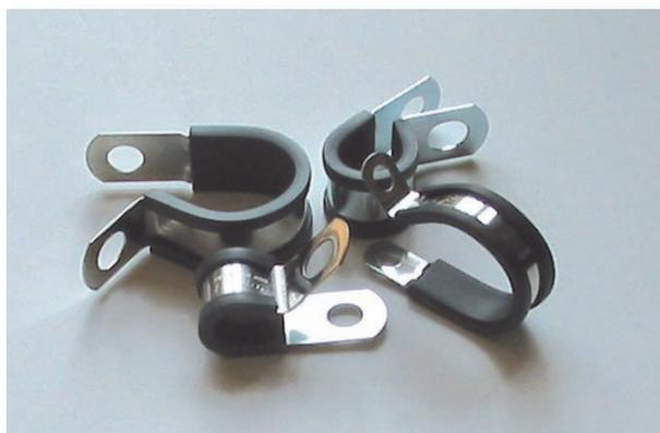
JCS P-CLIPS are available in two ranges for 6mm and 10mm bolts in both zinc-plated finish and 18/8 stainless steel. Two types of TPE liner with different service temperatures can be supplied.
