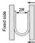
Note) At a temperature of 20°C bend the tubing into a U shape. Then with one side fixed, gradually close the other side and measure 2R at the point where the tubing folds or flattens, etc.
