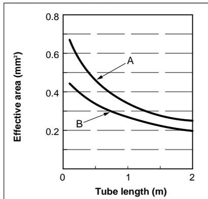
A : When the One-touch Mini (KJH02-M5) are connected to the ends of a straight tube.
