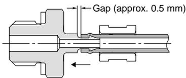
4. Insert the sleeve slowly. Make sure not to allow any gap between the sleeve end side and the body end side. (Please refer to the illustration below.)
