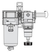
2. Do not allow twisting or bending moment to be applied other than the weight of the equipment.
