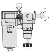
Piping materials without flexibility such as steel tube piping are prone to be effected by excess moment load and vibration from the piping side. Use flexible tubing in between to avoid such an effect.
