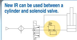
Note) The set pressure may vary depending on the elapsed time and change in ambient temperature after pressure setting. If the setting value varies, adjust the pressure with the knob.
