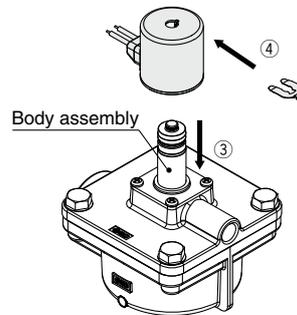
Step 2) Assemble the coil.
