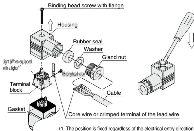
Internal connections are as shown below. Make connections to the power supply accordingly.
