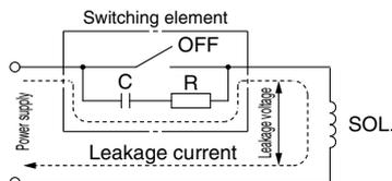
AC coil: 5% or less of rated voltage
