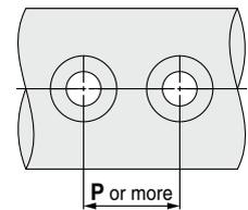
**Tank hole machining**
