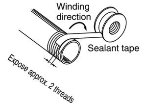
4. When using a fitting other than an SMC fitting
