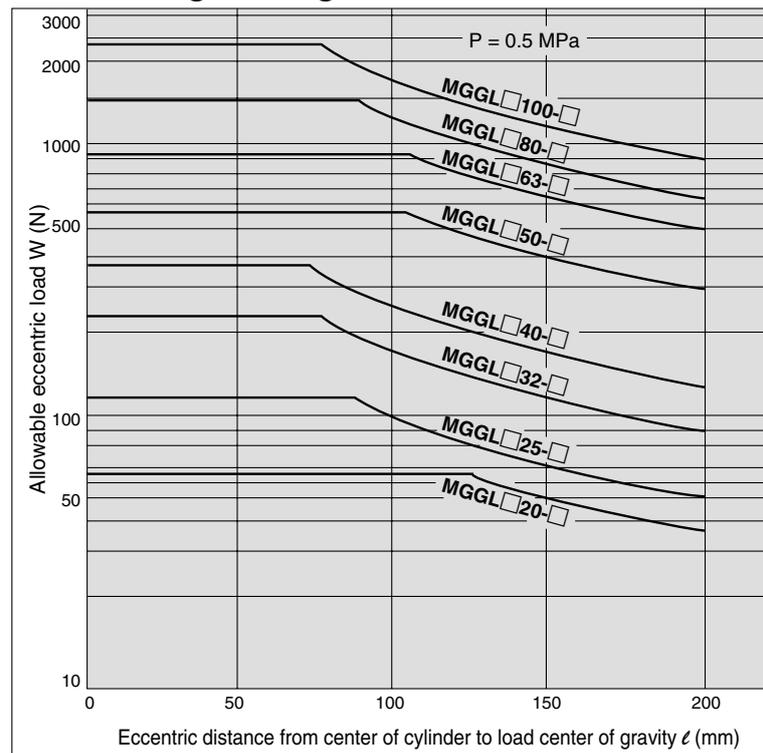
(Set the maximum allowable load so that it does not exceed the following percentages of the theoretical output: 40% for  $\phi 20$ , 50% for  $\phi 25$ , and 60% for  $\phi 32$ ,  $\phi 40$ ,  $\phi 50$ ,  $\phi 63$ ,  $\phi 80$  and  $\phi 100$ .)
