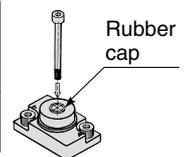
Remove the bolt for normal operation.
