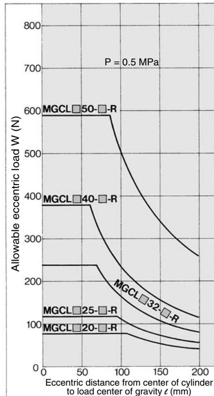
(Set the maximum allowable load so that it does not exceed the following percentages of the theoretical output: 40% for  $\phi 20$ , 50% for  $\phi 32$ , 55% for  $\phi 40$  and 60% or less for  $\phi 50$ , respectively.)
