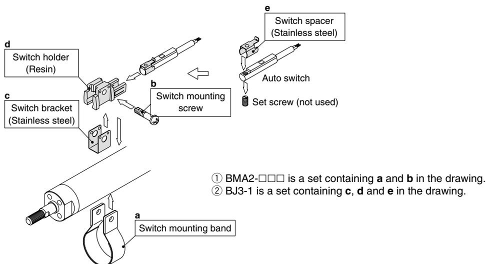
Other than the applicable auto switches listed in "How to Order", the following auto switches can be mounted. For detailed specifications, refer to SMC's "Best Pneumatics" catalogue, etc.
