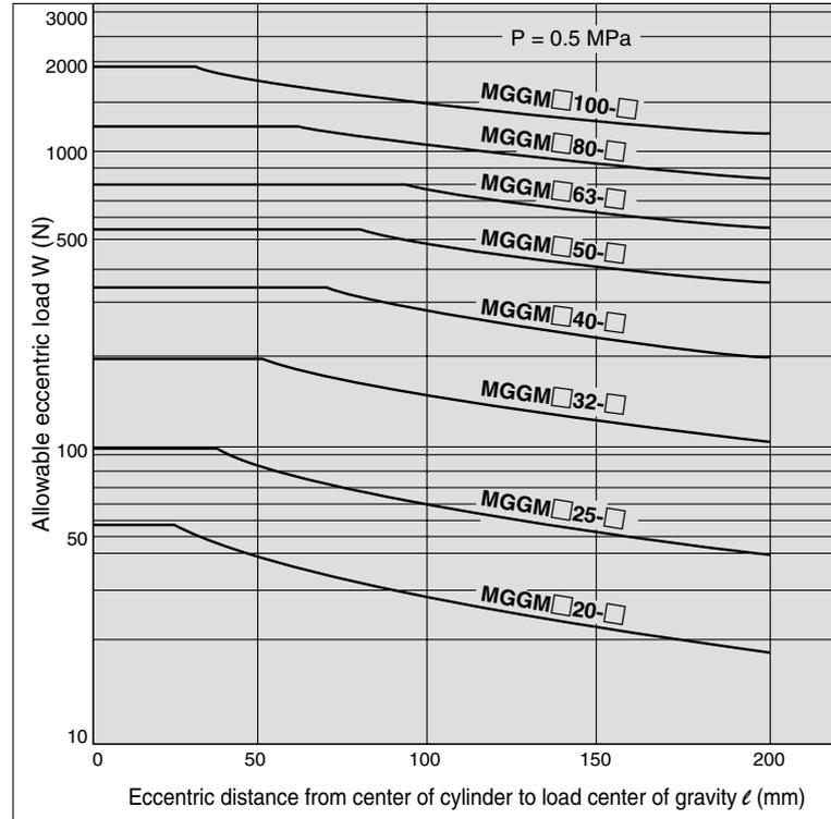
(Set the maximum allowable load so that it does not exceed the following percentages of the theoretical output: 35% for  $\phi 20$ , 40% for  $\phi 25$ , 50% for  $\phi 32$ , 55% for  $\phi 40$  and  $\phi 50$ , and 50% for  $\phi 63$ ,  $\phi 80$  and  $\phi 100$ .)
