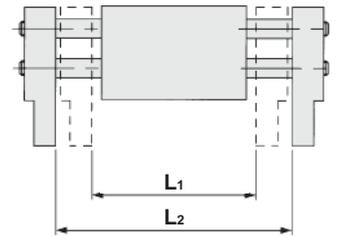
\* The opening and closing widths represent the value when gripping the exterior of a workpiece.
