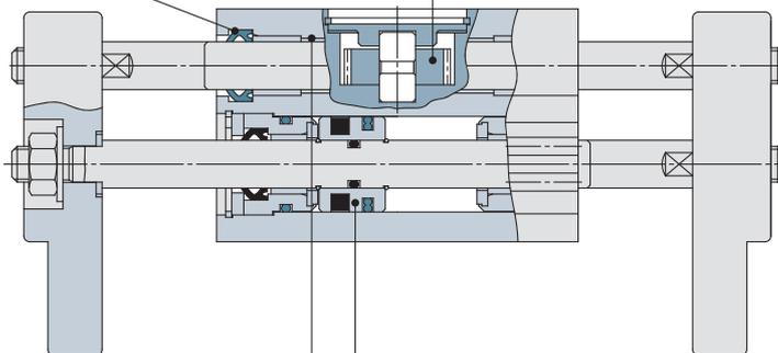
Double-end type oil-impregnated resin bearings are used for all shafts.
