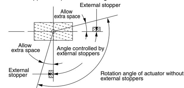
External stopper becomes a fulcrum, and load's inertial force is applied to shaft as bending moment.
