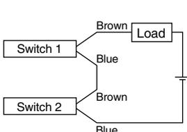
When two switches are connected in series, a load may malfunction because the load voltage will decline when in the ON state. The indicator lights will light up if both of the switches are in the ON state.
