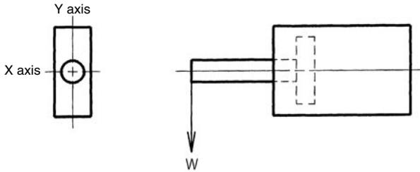
\* In the case of a plate cylinder, although there is the possibility that a load is applied in both X and Y axis as illustrated, the allowable lateral load is the same.
