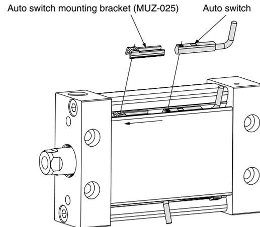
3. Confirm where the mounting position is, and tighten the auto switch mounting screw using a flat head screwdriver to fix the auto switch.
