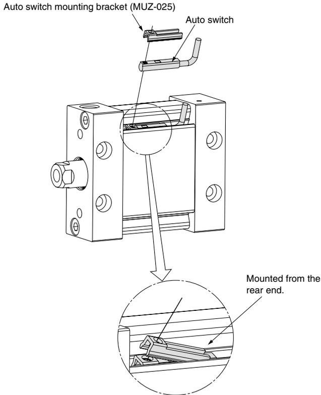
\* The auto switch mounting bracket should be mounted from the rear end.
