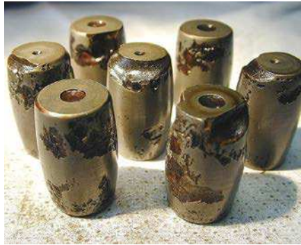
Rollers from a counterfeit spherical roller bearing
