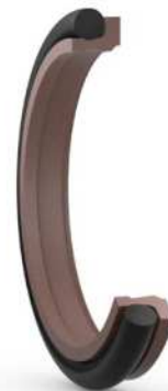
Double-acting wiper A27-F with o-ring as energizer made of SKF Ecoflon 3 and NBR 70
