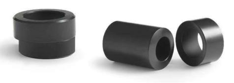
Spherical washers from SKF are designed to create an exact parallel plane between the bolt head and the face of the nut. This spherical washer automatically adjusts to compensate for angle errors and eliminate bolt bending.
