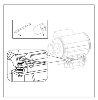
Tighten the foundation bolts in the sequence and number of runs given by the Original Equipment Manufacturer (OEM).
