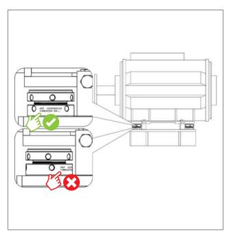
Install the SKF Vibracon chock in a position that it is easy to read the batch number. Location of the batch number faced to the outside of the installation is preferred.
