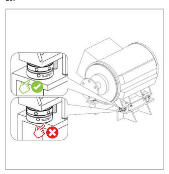
The bottom ring of the SKF Vibracon chock should be completely, 100%, supported by the support construction.
