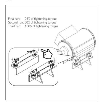
In case the number of runs is not given by the OEM, SKF recommends tightening the bolts in a minimum of 3 runs.
