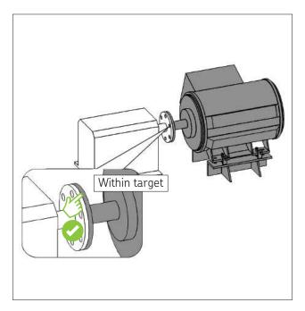
Check if the alignment of the component is within the tolerance of the final alignment target.
