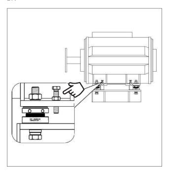
After the alignment check the vertical adjustment bolts can be locked with a hexagonal nut.
