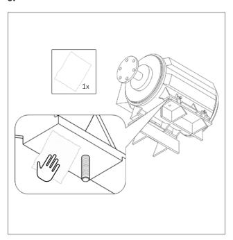
Clean the lower side of the base plate (foot) of the component with a cloth.
