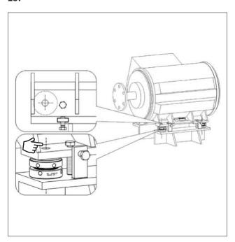
Center the position of the SKF Vibracon chock concentric with the bolt hole.
