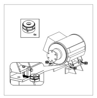
Insert the SKF Vibracon chock from the side at the foundation bolt hole positions.
