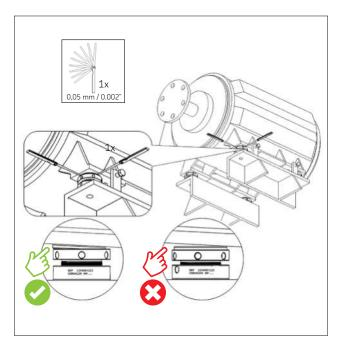
The SKF Vibracon top plate needs to be in contact with the bottom side of the component foot.
