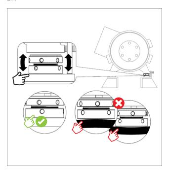
Execute a so-called wobbling / rocker test to check the quality of the contact surface between SKF Vibracon chock and support construction.
