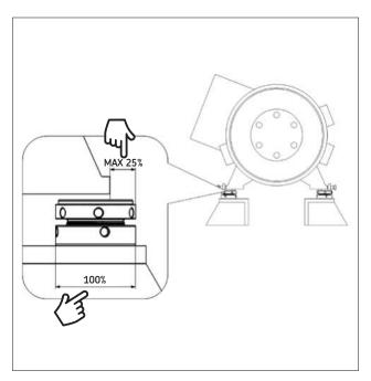
The top plate of the SKF Vibracon chock should be covered by the component foot by at least 75%.
