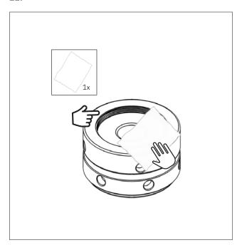
Advice is to clean the bottom of the SKF Vibracon chock with a clean cloth.
