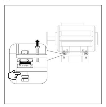
Release the adjustment bolts, the complete weight of the component is now transferred unto the SKF Vibracon. The foundation bolts are not to be tightened before releasing the adjustment bolts!
