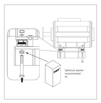
Install the foundation bolt, preferably from bottom up. SKF recommends the use of the SKF Spherical washer.
