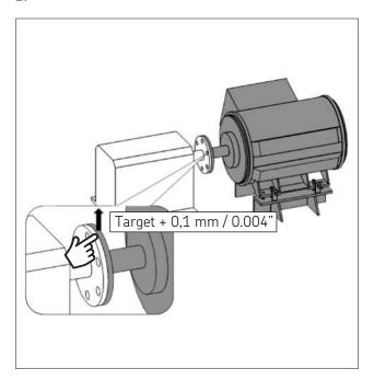
For compensation of compression of the total chocking package during tightening of the foundation bolt it is advised to position the component 0.1 mm (0.004 inch) above target.
