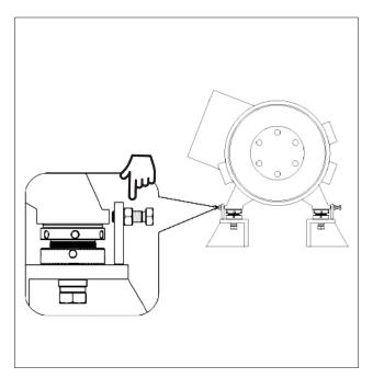
After finalizing the alignment, lock the horizontal adjustment bolts with a hexagonal nut.
