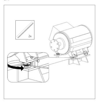
Adjust the center ring by using two rods which fit in the circular holes in the outer circumference of the center ring and the bottom ring.
