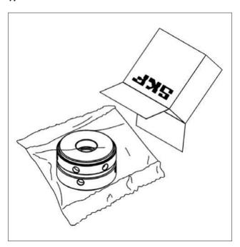
The SKF Vibracon chock is packaged in a corrosion protective plastic bag.
