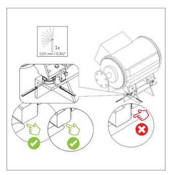
Check the flatness / contact area using a feeler gauge of 0.05 mm (0.002 inch).
