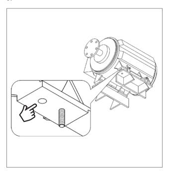
Visual inspection of the lower side of the base plate. Surface should be free from damages, dirt and rust. Paint is not preferred and can have an influence on the clamping force of the foundation bolt!
