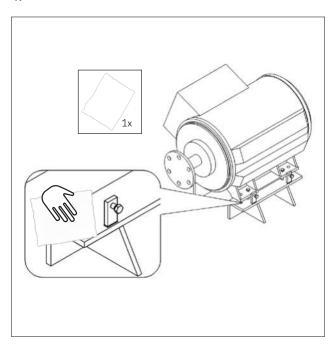
Clean the top side of the top plate of the support construction with a cloth.
