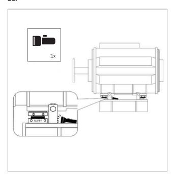
From field experience we advise to make use of a flashlight for an easy check of the contact areas between the SKF Vibracon chock and the component.
