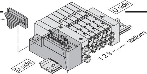
\* Valves are numbered from the D side.
