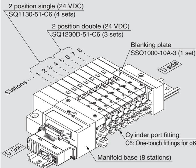
SS5Q13-SB08-D ..... 1 set (SB kit 8-station manifold base part no.)
