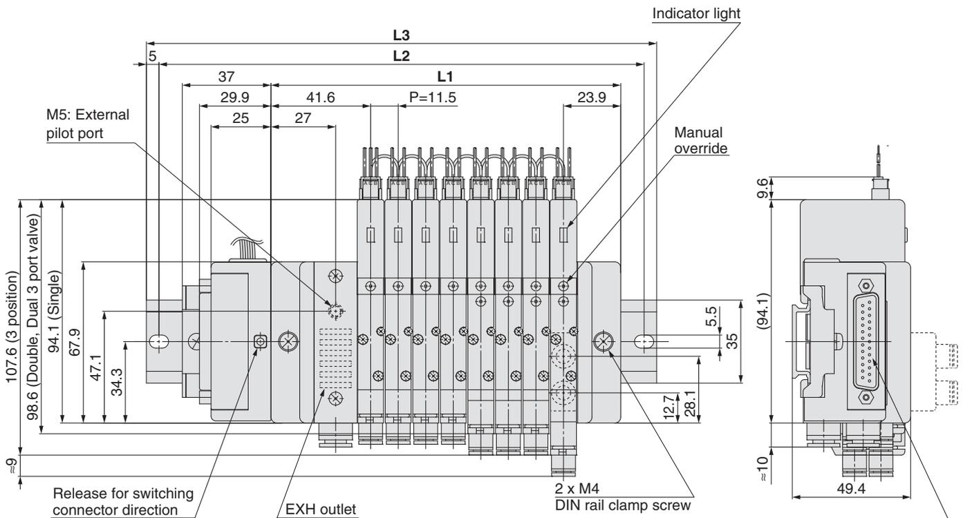
Applicable connector: D-sub connector (25P)
