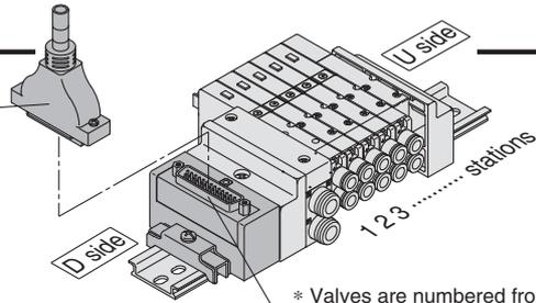
\* Valves are numbered from the D side.
