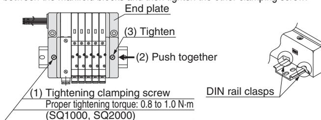
Confirm that the DIN rail clasps are securely hooked into the DIN rail.
