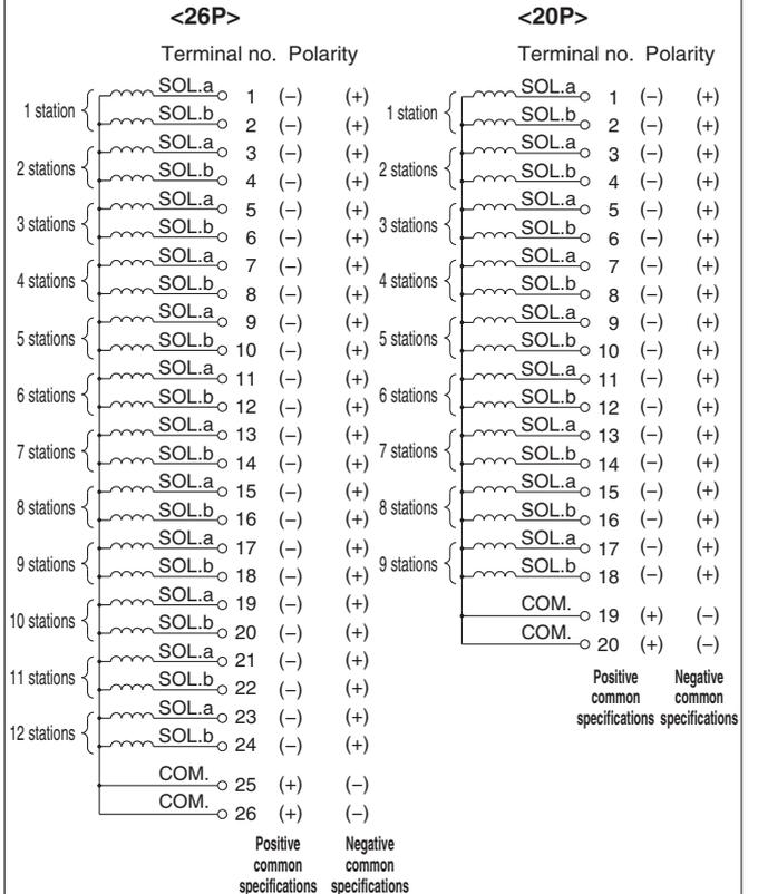
Note) When using the negative common specifications, use valves for negative common.
