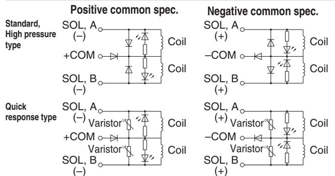
Note) With quick response type, approximately -40 V of coil surge voltage is generated when the valve is switched OFF.
