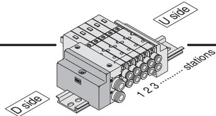
\* Valves are numbered from the D side.
