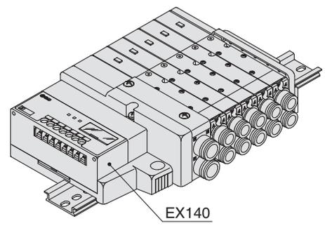
Refer to catalogue and the Operation Manual for the details of EX140 integrated-type (for output) serial transmission system. Please download it via our website, <http://www.smc.eu>
