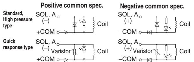
Note) With quick response type, approximately -40 V of coil surge voltage is generated when the valve is switched OFF.
