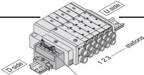
\* Valves are numbered from the D side.
