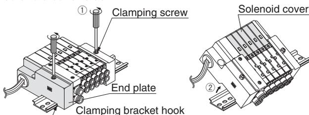
When a manifold contains a large number of stations and it is difficult to remove all at once, separate the manifold into several sections before removing it.
