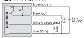
Max. load current: 80 mA, Internal voltage drop: 1.5 V or less
