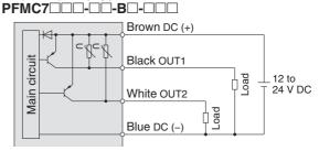
Max. load current: 80 mA, Internal voltage drop: 1.5 V or less
