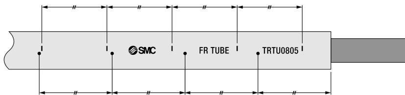
Strip off the aluminium laminated film to prevent the inner tube from being damaged.
