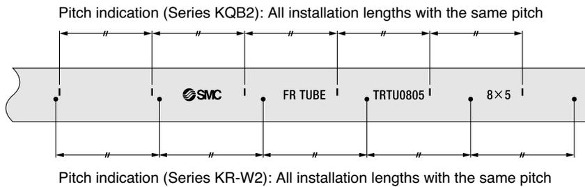
**Identification of the pitch length for installation**
