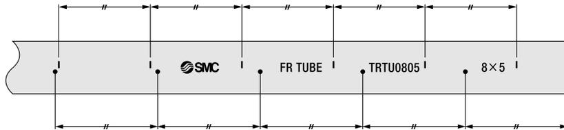
Outer layer, aluminium laminated film and inner tube are cut at the “•” mark.
