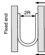
Bend the tube into U-form at the temperature of 20°C. Fix one end and close loop gradually. Measure 2R when the tube breaks or is crushed.
