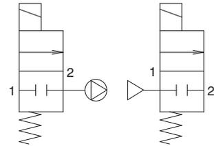
Note) The configuration symbol shows ports 1 and 2 as blocked, but there is actually a limit to the blocking capability when the pressure of port 2 is greater than the pressure of port 1. Please contact SMC when low leakage performance is required.
