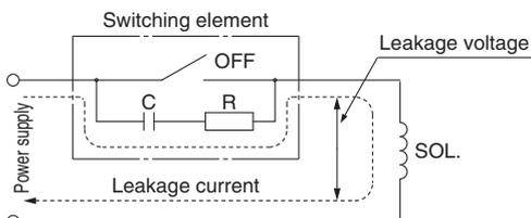
AC/Class B built-in full wave rectifier coil: 10% or less of rated voltage
