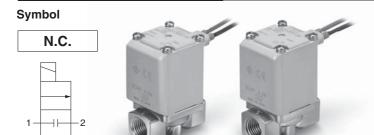
When the valve is closed, flow is blocked from port 1 to port 2. However, if the pressure in port 2 is higher than port 1, the valve will not be able to block the fluid and it will flow from port 2 to port 1.
