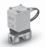
When the valve is closed, flow is blocked from port 1 to port 2. However, if the pressure in port 2 is higher than port 1, the valve will not be able to block the fluid and it will flow from port 2 to port 1.
