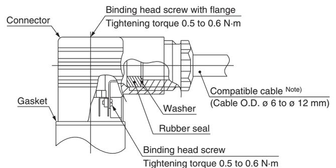
Note) For an outside cable O.D.  $\phi$  9 to  $\phi$  12 mm, remove the internal parts of the rubber seal before using.
