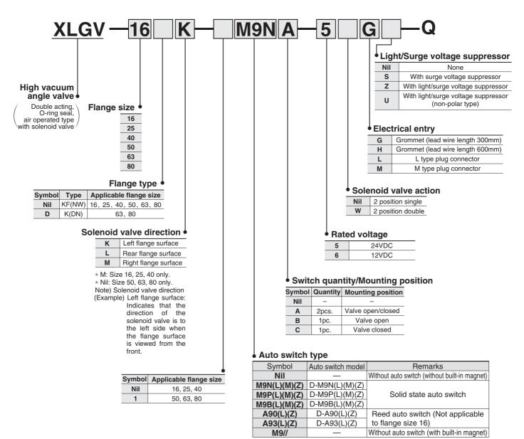
Standard lead wire length is 0.5 m. Add "L" to the end of the part number when 3 m is desired, "M" when 1 m, and "Z" when 5 m. Example) -M9NL  $\_$
