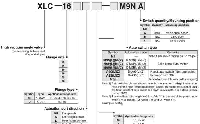
Right flange surface Note) Actuation port direction (Example) Left flange surface: Indicates that the direction of the actuation port is to
