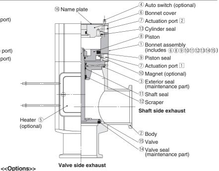
4 Auto switch: The magnet (10) actuates the auto switch (4) indicating the position of the integrated valve (15) and piston (8). With 2 auto switches, the open and closed positions are detected, and with 1 auto switch, either the open or closed position is detected. Auto switches are applicable at ordinary temperatures only (5 to
