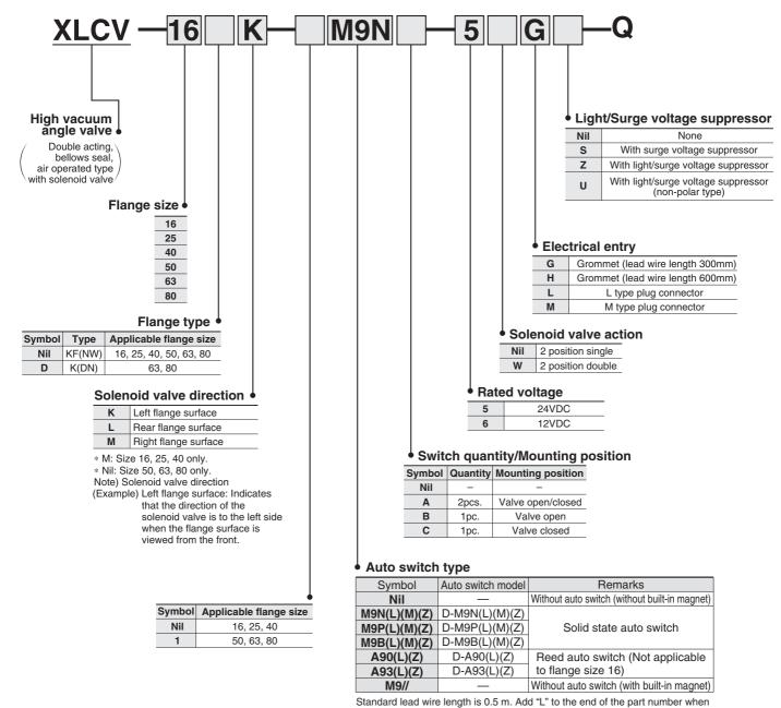
3 m is desired, "M" when 1 m, and "Z" when 5 m. Example) -M9NL
