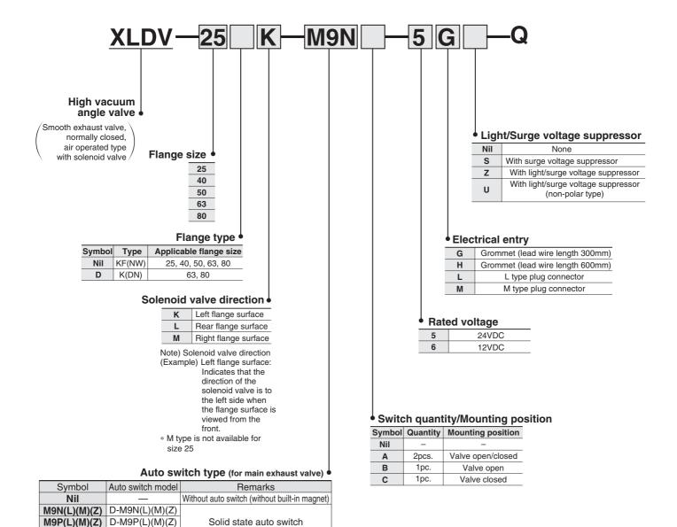
Standard lead wire length is 0.5 m. Add "L" to the end of the part number when 3 m is desired, "M" when 1 m, and "Z" when 5 m. Example) -M9NL  $\_$
