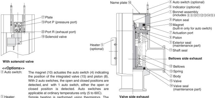
Simple heating is performed using thermistors. The valve body can be heated to approximately 80, 100 or 120C, depending on the heater option and the valve size. The type and number of thermistors to be used will vary depending upon size and setting temperature. In the case of high temperature specifications, the bonnet assembly (1) is a heat resistant structure.
