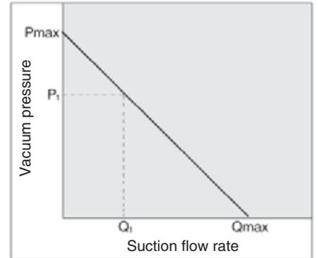
Flow characteristics are expressed in ejector vacuum pressure and suction flow. If suction flow rate changes, a change in vacuum pressure will also be expressed. Normally this relationship is expressed in ejector standard supply pressure. In graph, Pmax is max. vacuum pressure and Qmax is max. suction flow. The values are specified according to catalog use.
