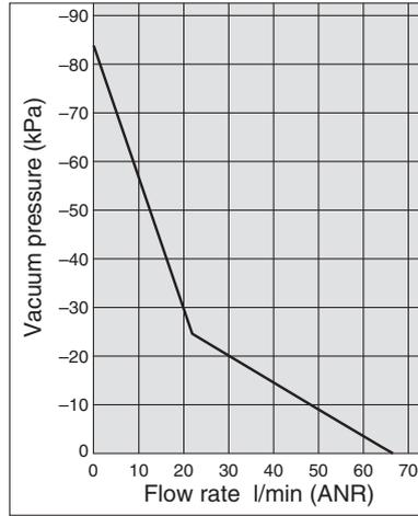
**Exhaust Characteristics/Flow Characteristics, Standard Supply Pressure: S ... 0.45 MPa**
