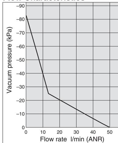
**Exhaust Characteristics/Flow Characteristics, Standard Supply Pressure: H ... 0.5 MPa**
