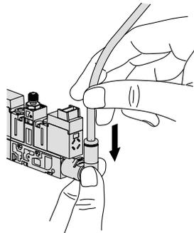
Especially if load is applied in the bending direction against the axial direction of the filter case, the case may be broken.
