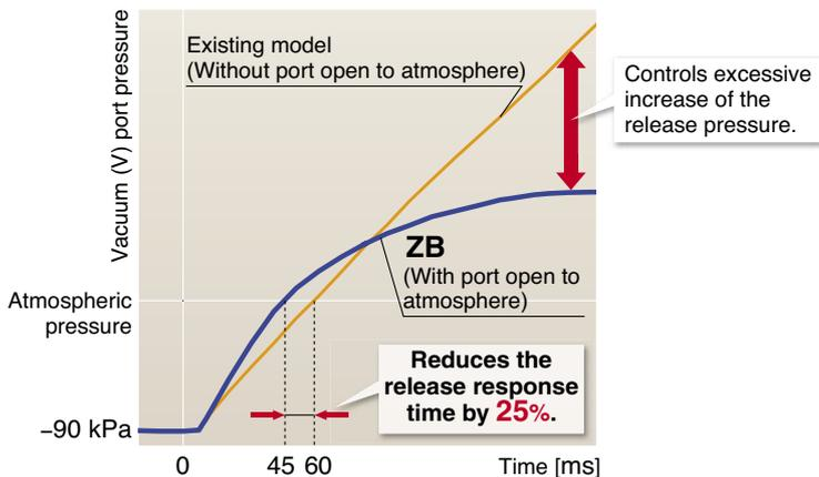
\* Conditions: Needle flow rate set to 5 L/min, with supply pressure 0.5 MPa, vacuum piping size  $\phi 4/\phi 2.5 \times 100$  mm
