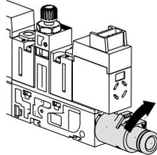
2. If it is mounted on the floor, remove the manifold base once from the installation position and lift the body to perform mounting and removal work so that the mounting and removal work can be performed more easily.
