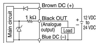
Voltage output type: 1 to 5 V
