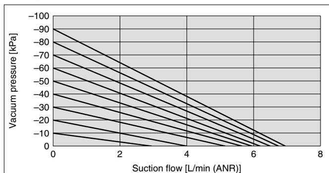
The actual suction flow at the point of suction varies depending on the vacuum pump's piping conditions. (For above graph, vacuum (V) port is  $\phi 4 \times 50$  mm.)
