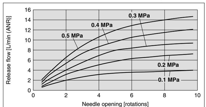
Note) The flow-rate characteristics shown in this graph are representative values, and the flow at the absorption part may vary depending on the piping conditions to the vacuum (V) port, etc.
