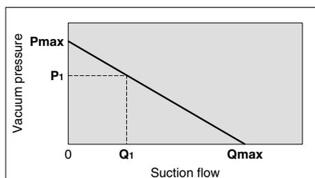
Flow-rate characteristics are expressed in ejector vacuum pressure and suction flow. If suction flow changes, the vacuum pressure will also be changed. Normally this relationship is expressed in ejector standard operating pressure use. In graph, **Pmax** is max. vacuum pressure and **Qmax** is maximum suction flow. The values are specified according to catalogue use. Changes in vacuum pressure are expressed in the below order.
