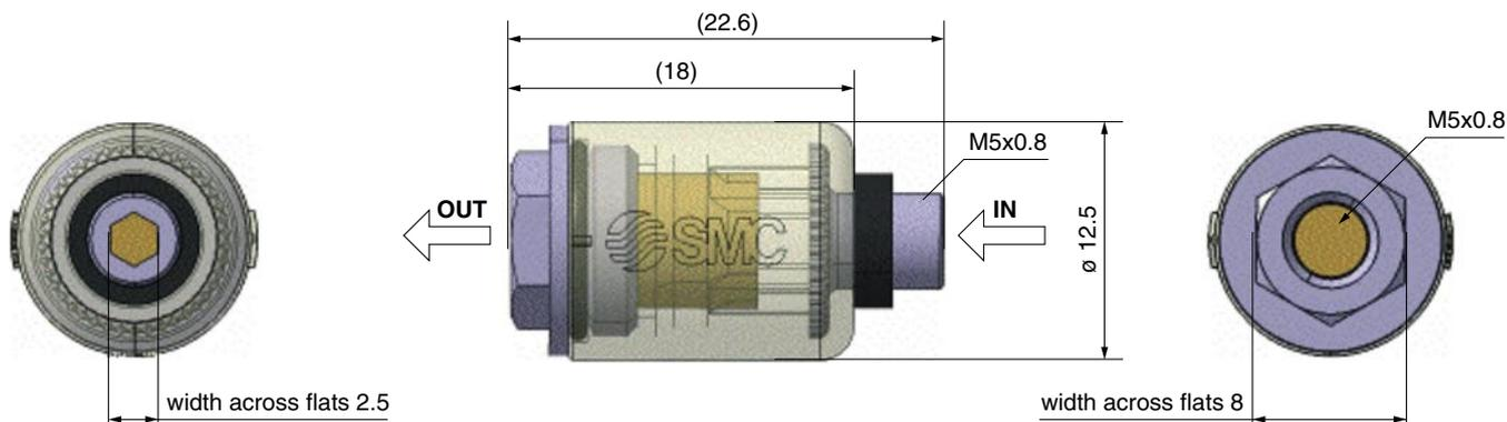
Note 1: Use is possible even with IN-OUT reversed-connection.
