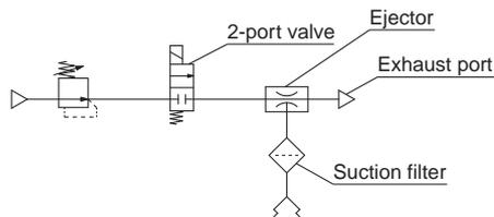
2-port valve is used to generate and stop the vacuum. Vacuum is released to the atmosphere. A suction filter is installed to protect the ejector.
