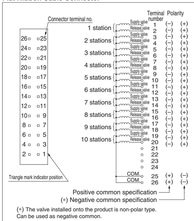
A flat ribbon cable connector (26P) conforming to MIL standards is used.
