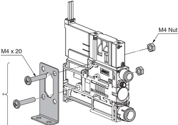
\*Mounting bracket for single unit (Option), [Nuts and bolts are included.]
