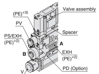
\*1) For models without valve, pressure can be 0.3 MPa or less.
