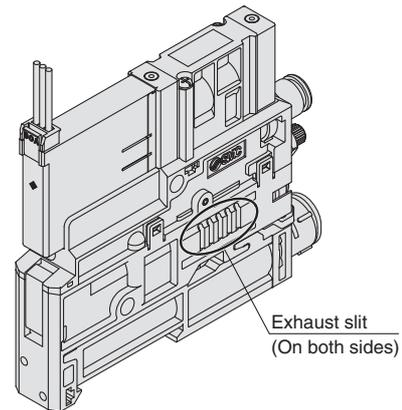
For port exhaust type, back pressure may increase depending on the piping size and length. Ensure that the back pressure does not exceed 0.005 MPa (5 kPa).
