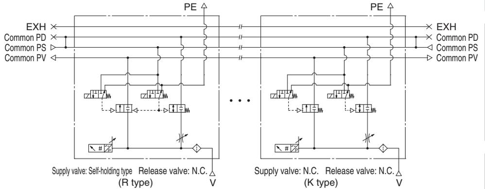
Supply valve: Self-holding type Release valve: N.C. (R type)
