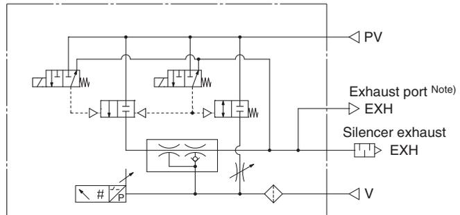
Supply valve: Self-holding type Release valve: N.C. (R type)
