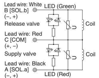
Light/surge voltage suppressor circuit is equipped for both single and double solenoid. Red LED turns on when supply valve (SOL.a) is energised. Green LED turns on when release valve (SOL.b) is energised.
