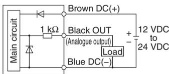
Voltage output type: 1 to 5 V
