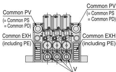
Note) The complex exhaust is a combined exhaust method of the common exhaust from the end plate and the direct exhaust from each station.
