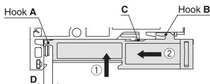
Note) If excess force is applied to the filter case, hook A and B may break. Handle with care.
