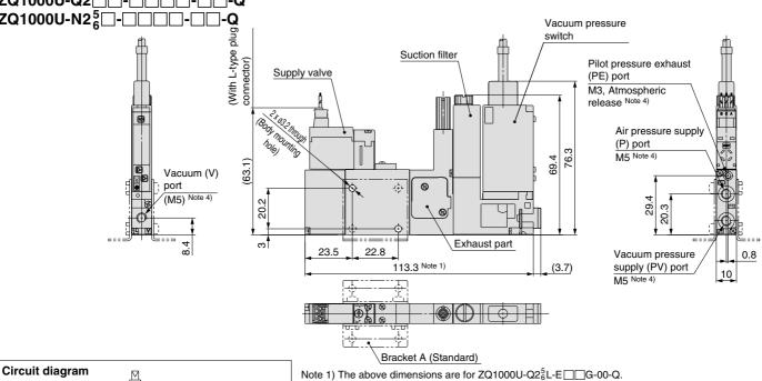
In case of ZQ1000U-Q2 \_\_\_-F-00-Q, the overall length is 87.2 Note 2) The dimensions after bracket A is mounted are the same as those of the K1 type.
