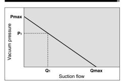
Flow characteristics are expressed in ejector vacuum pressure and suction flow. If suction flow rate changes, a change in vacuum pressure will also be expressed. Normally this relationship is expressed in ejector standard use.
